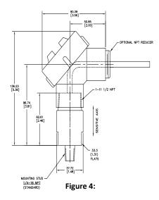
Figure 4: Outline dimensions of the SW5484E Flying Lead Version. Dimensions in mm [inches]. 8200-000 IEC conduit elbow shown installed, necessary for Explosion Proof rating.
