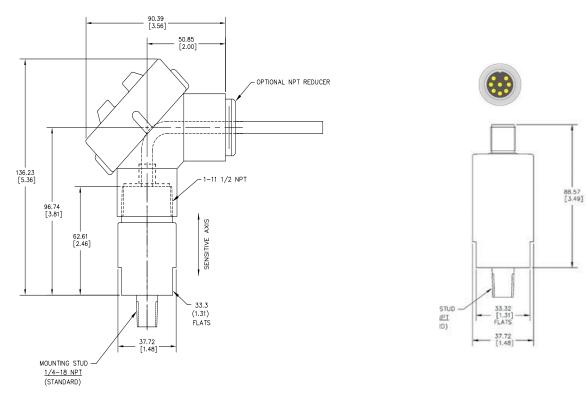
Figure 1: Outline dimensions of the SW5484E Flying Lead Version. Dimensions in mm [inches]. 8200-000 IEC conduit elbow shown installed, necessary for Explosion Proof rating.
